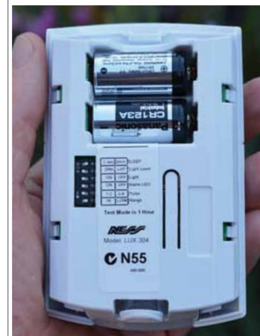
Rear of sensor with battery case and settings
